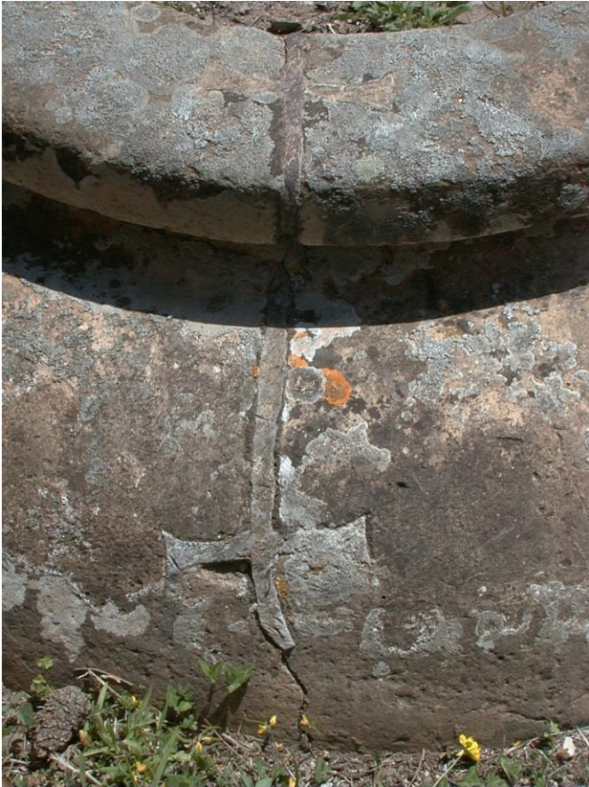
Figure 2: Dolium with dunting crack repaired with lead filler and two lead clamps. Second century AD. Caseggiato dei Doli, Ostia Antica, Italy.
